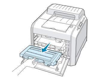
**CAUTION**: If you open the left cover for a few minutes, the imaging unit can be exposed to light. This causes damage to the imaging unit.
